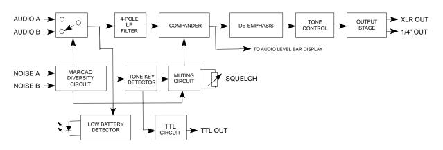
Figure 2. UC4 Audio Section Block Diagram
