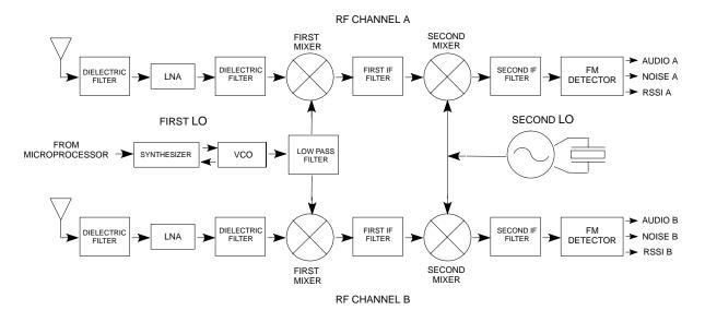
Figure 3. UC4 Rf Section Block Diagram
